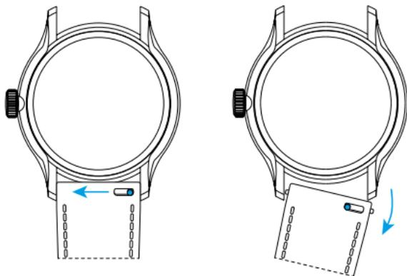
1. Locate the quick-release pin on your strap. Pull the pin to the side to detach your strap.
