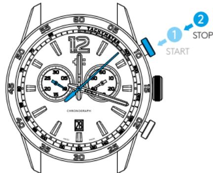
To stop the timing, press push-button A once more and read the 2 chronograph counters, for example: 2 hours/10 mins/8 seconds.
