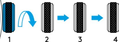
For a superior water resistance your crown is of the screw-in type. The crown should sit flush to the case (position **1**) in order to maintain water resistance.
