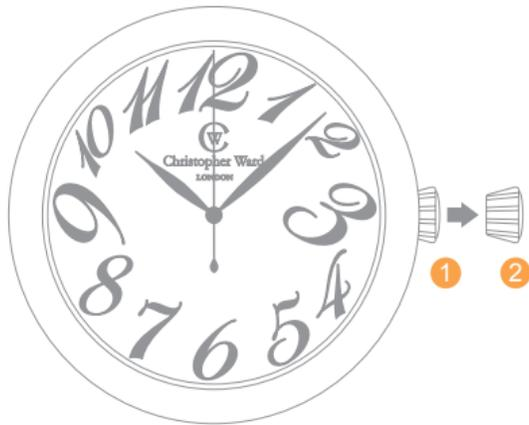
Pulling the crown out to position ②, stops the secondhand
