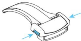
2. Pull open the clasp and locate the opening.
