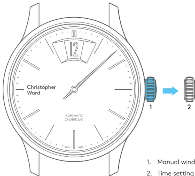
The crown should sit flush to the case (position 1) in order to maintain water resistance.
