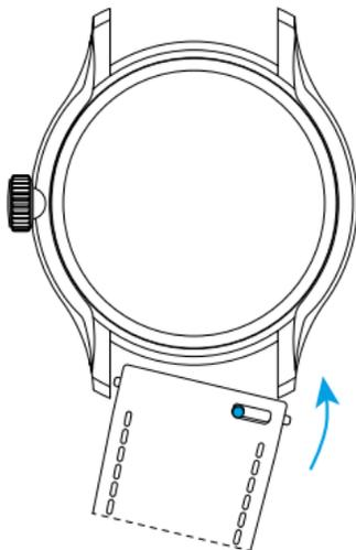
2. To reattach your strap, align the pins to the lug holes and click the strap into position.
